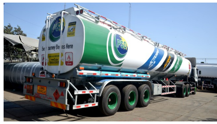
48,000 Liters, 4 Compartment, Fuel Tank Tanker PSO Standard.
