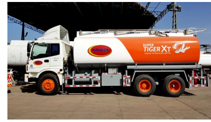
20,000 Liters, 3 Compartment, Fuel Tank Tanker Hascol Standard
