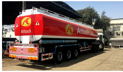
48,000 Liters, 5 Compartment, Fuel Tank Tanker APL Standard
