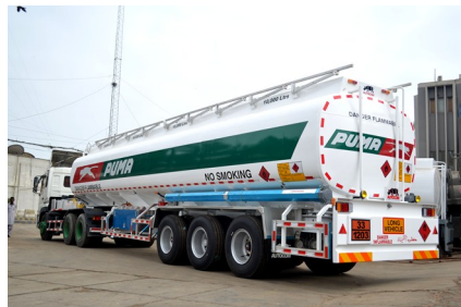
48,000 Liters, 5 Compartment, Fuel Tank Tanker PUMA Standard
