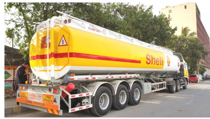
48,000 Liters, 3 Compartment, Fuel Tank Tanker With EBS and Bottom Loading Shell GVS Standard.
