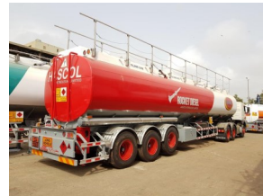
50,000 Liter Tanker Hascol Standard with Air Suspension
