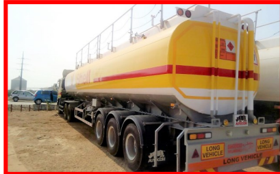
48,000 liter fuel tanker, 3 compartment, Shell GVS Standard
