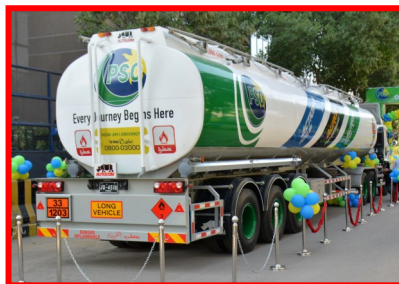
48,000 Litres Fuel Tanker, 4-Compartment, PSO Standard
