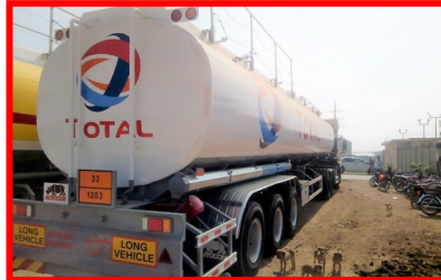
48,000 liter fuel tanker, 4 compartment, Total PATROM Standard
