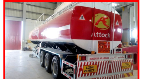
48,000 liter fuel tanker, 5 compartment (APL Standard)
