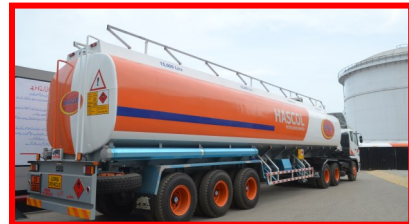
50,000 Liters Fuel Tanker, 4-Compartment, Hascol Standard
