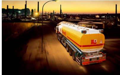
48,000 liter fuel tanker, 3 compartment, Shell GVS Standard
