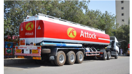
48,000 liter fuel tanker, 5 compartment (APL Standard)
