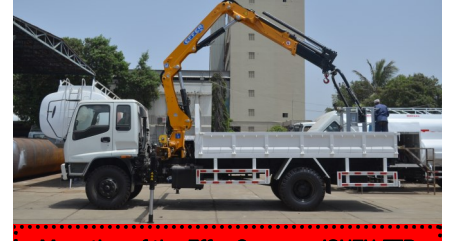
Mounting of the Effer Crane on ISUZU FTR truck chassis with cargo body
